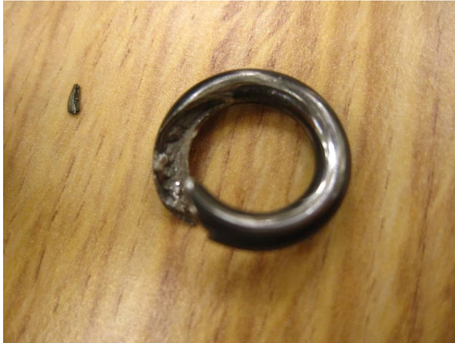
Figure 8. Fatigue Failure of a Spring.
