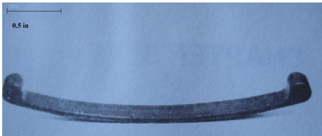
Figure 2 Leaf Spring (courtesy of Tubal Cain).
